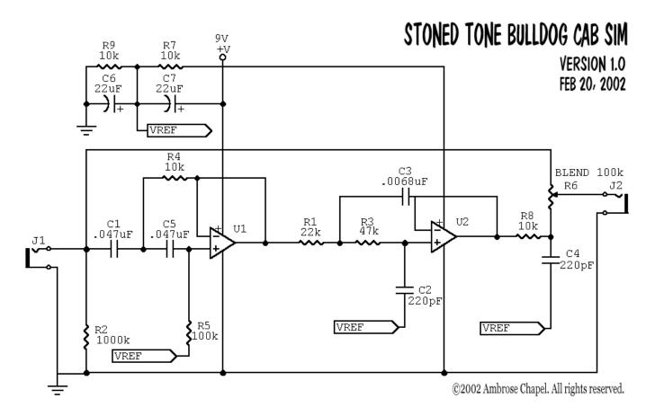
Bypass switching etc isn't shown or needed depending on your application. Just one control - "Blend", a linear pot. It blends between the straight signal and the cab sim.
